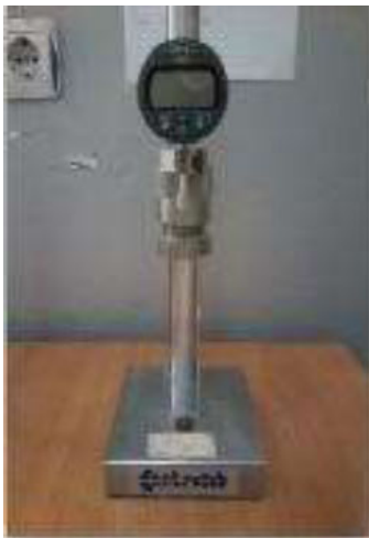
Fig. (6). Frame to measure shrinkage deformation.
