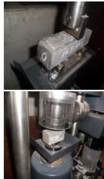
Fig. (3). Flexural and compressive strength test.
