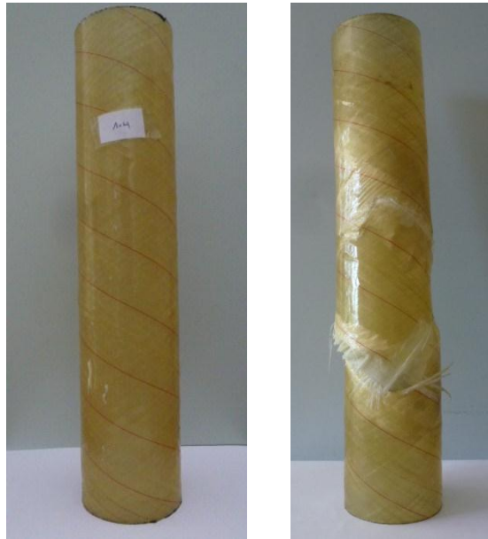
Fig II.23. Epoxy /glass composite tube before and after a tensile test
