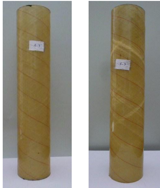
Fig II.17. Epoxy /glass composite tube before and after a tensile test
