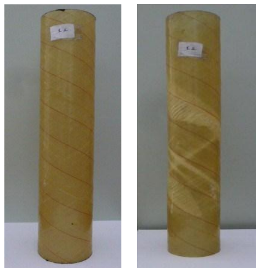
Fig II.11. Epoxy /glass composite tube before and after a tensile test
