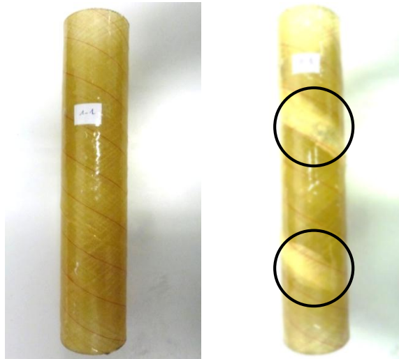
Fig II.9. Epoxy /glass composite tube before and after a tensile test.
